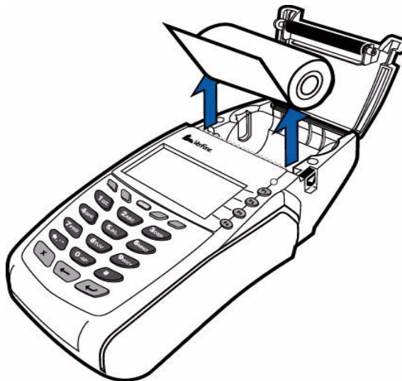
Figure 8 Removing Partial Paper Roll
