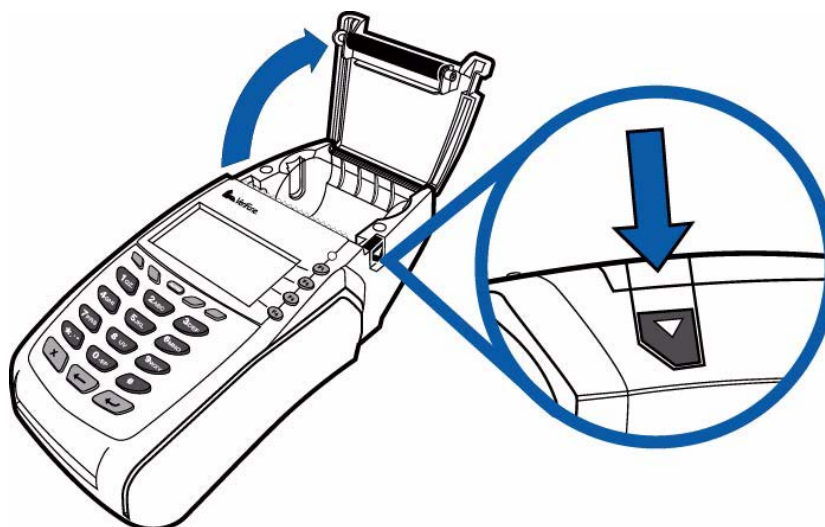
Figure 7 Opening the Printer Cover
