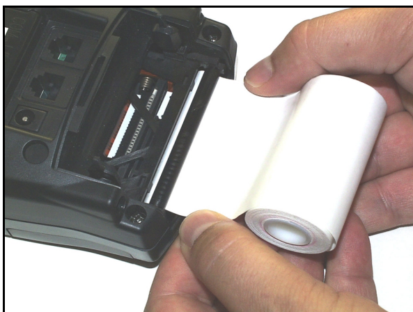
Figure 2-6. Loading the paper roll
