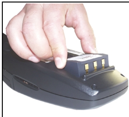
Figure 2-3. Installing the ICE 4000 Battery Pack
