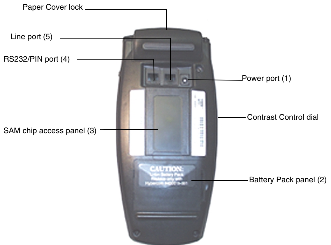
Figure 2-8. ICE 4000 under panel connectors
