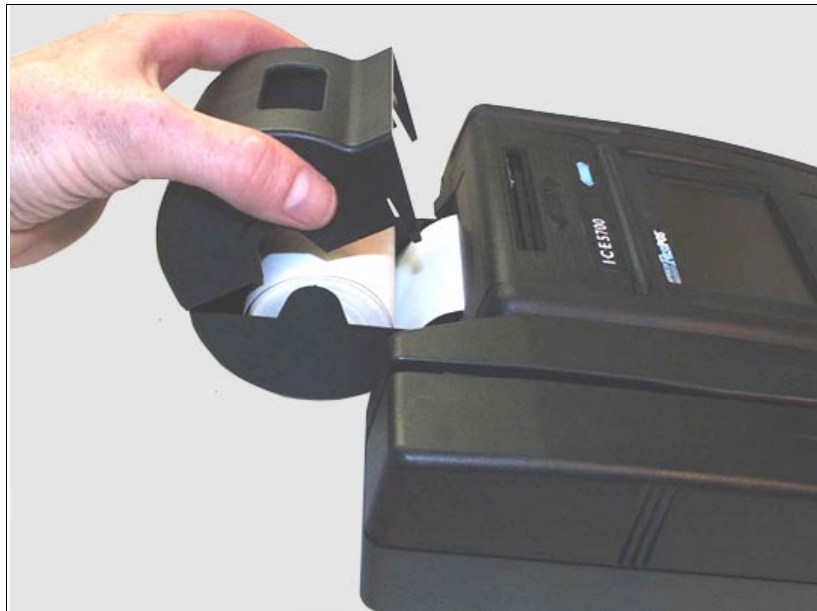
Figure 3-1. ICE 5700 printer paper door open
