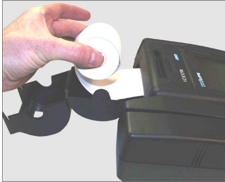
Figure 3-2. ICE 5700 printer paper installation
